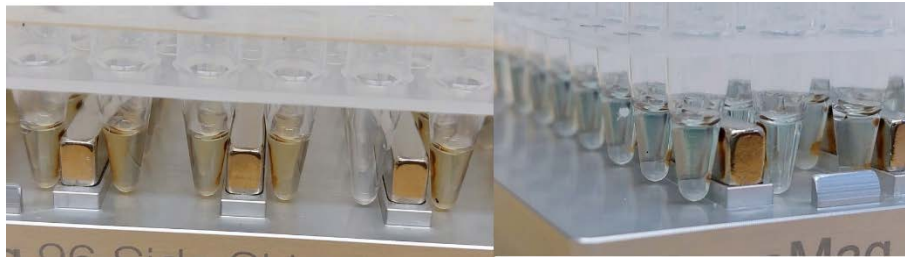
Figure 4. Bead mixture on magnetic stand. Left: mixture is not yet entirely clear and still a bit yellowish. Right: Mixture is clear, and the blue color of indexes added in the previous step can be seen.
