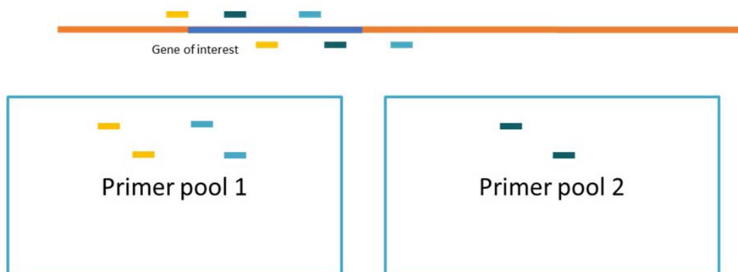
Figure 2. Overlapping amplicon design and primer pools. In order to allow for amplification of large genes, the custom DNA panel includes short overlapping amplicons. By using two pools of primers alternating the overlapping amplicons, we prevent amplification of the wrong primer combination in the overlapping region. After the initial two PCR reactions with the two primer pools, you add both products together and continue with a single library preparation in the next step.
